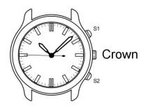
S1 Button is at 2 o'clock (outward) S2 Button is at 4 o'clock (inward)
